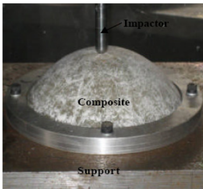
Figure 4. Impacted composite dome.
