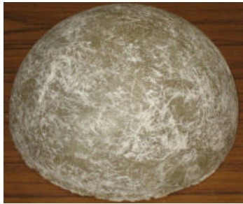
Figure 1. Photograph of manufactured 150mm diameter composite.
