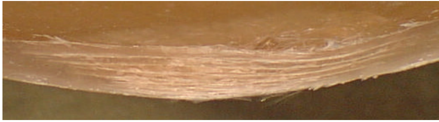
Figure 9. Through the impact point sectioned macro-photograph damaged composite dome.
