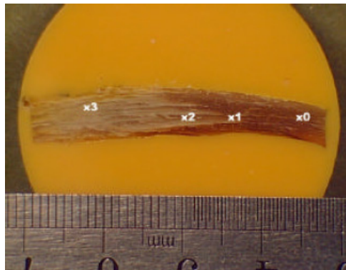
Figure 10. Sectioned composite impregnated in a resin for micro-photographs.
