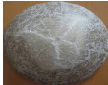
Figure 8. Damaged 200mm diameter composite dome due to impact.
