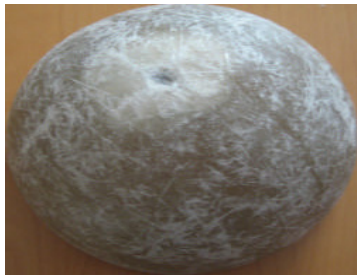
Figure 7. Damaged 150mm diameter composite dome due to repeated impact.
