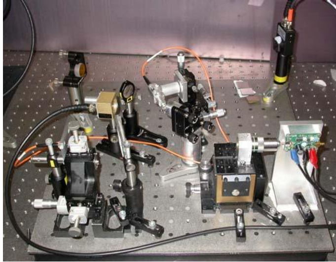
Figure 4. (Color online) Apparatus used for 850nm pumped VCSEL experiment.
