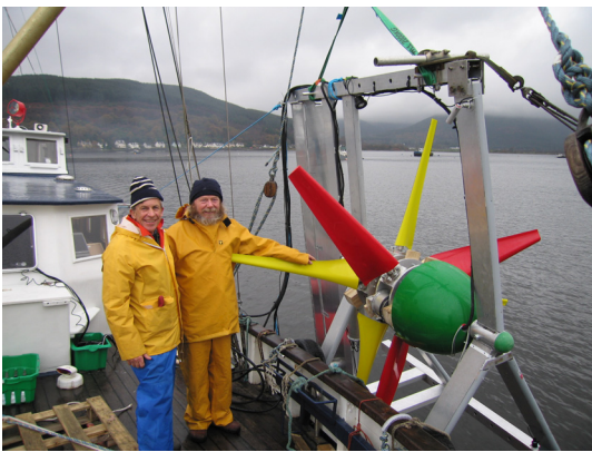
Figure 12: CoRMaT on frame aside the St Hilda (nacelle cowling removed)
