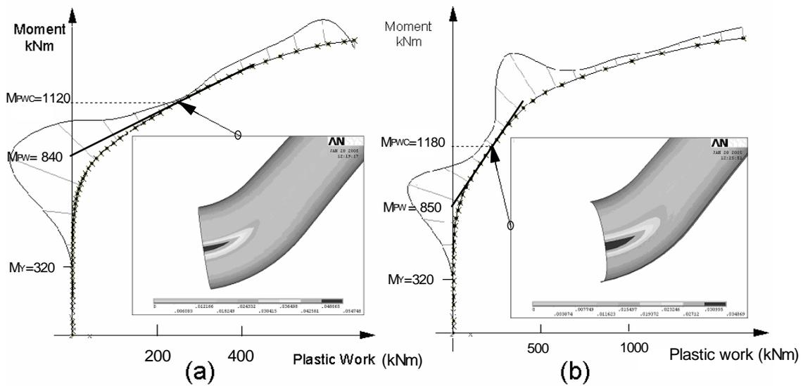
Figure 8. Opening moment large deformation analysis (a) perfectly plastic (b) 2% bilinear hardening, with von Mises equivalent plastic strain contour plots at specified PWC plastic load.
