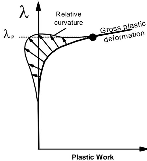
Figure 3. Plastic Work Curvature, PWC, criterion.
