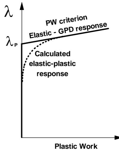
Figure 11. Plastic Work criterion elastic-GPD response model.
