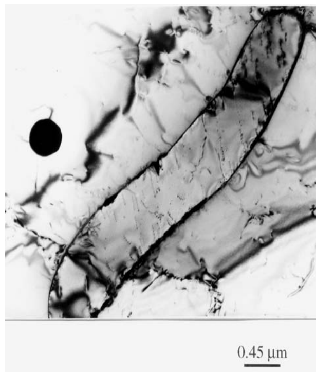
Figure 7 TEM Bright field micrograph showing delta ferrite with slight precipitation on the \delta/\gamma grain boundary, in specimen C9, weld T15.
