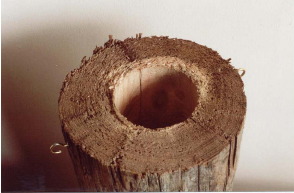
Figure 7 Short pole section showing cup hooks and 75 mm central “decay” hole.
