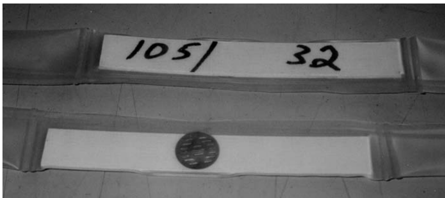
Figure 1: Metastable composite specimens exhibiting the disc used to initiate crystallisation and flexible PVC film containment.
