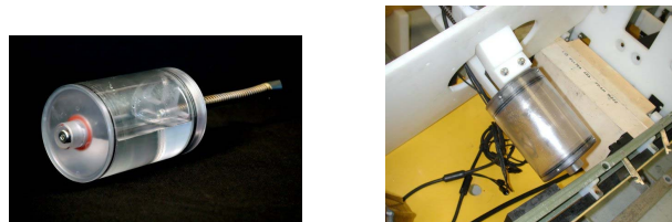
Fig. 1. The Gulper water-sampling device and its mounting inside an AUV mid-section.
