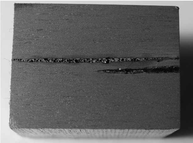
Figure 12: Forging No. 447 660. Macro-shape of the sample at the place of defect location. Slika 12: Odkovek št. 447 660. Vzorec z mestom napake.
