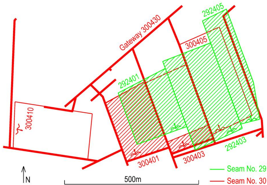
Fig. 7. The situation of mine workings and mining before the failure of the whole rigid overlying strata.
