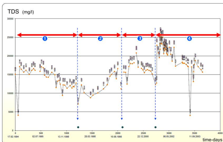
Fig.4 Development of TDS in the mine water of the shaft Jeremenko (the Upper Silesian Coal Basin – Ostrava part [7])
