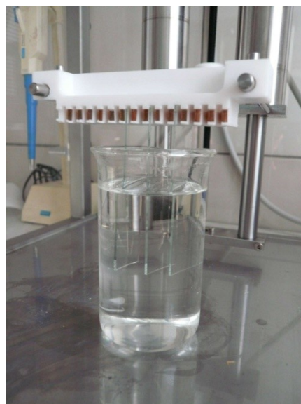
Fig.17 The dip coating of glass plate into the \text{SiO}_2 -B sol.
