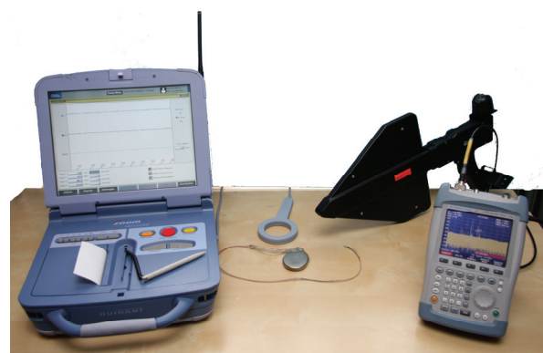
Fig. 8. Measuring workplace for electromagnetic RF disturbing signals influence
