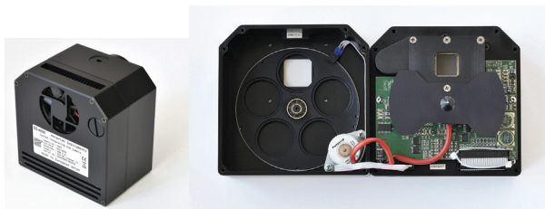
Fig. 3. Ventilator location for cooling Peltier cells and interior of CCD camera with disc for 5 filters
