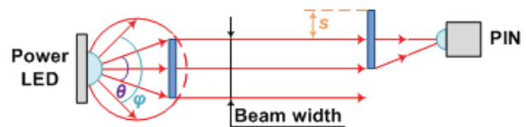
Fig. 6. Repositioning of the receiving part by the parameter s according to fig. 4
