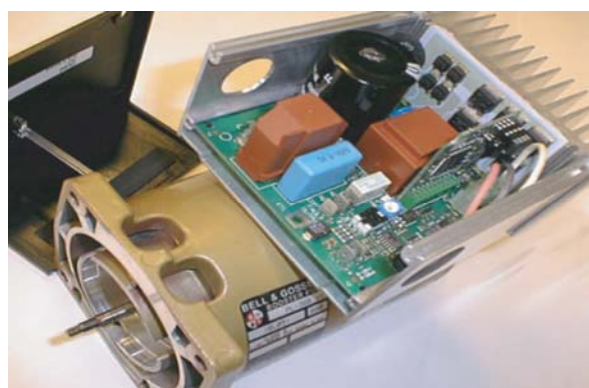
Fig. 1. Two-phase drive using voltage inverter and 3-phase low-cost motor [4]
