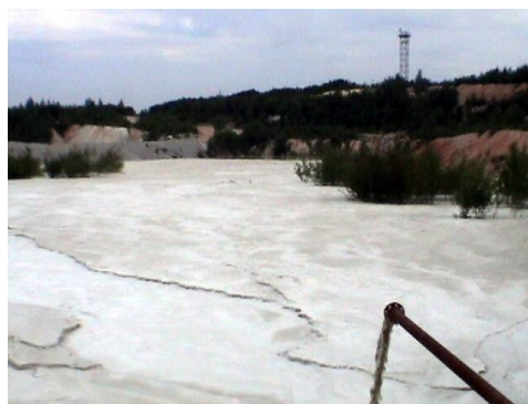
Pic. 1 Subaerial tailings discharge (after processing of kaolin)
