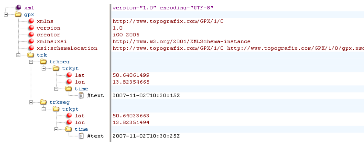
Fig. 1 XML scheme of GPS file
