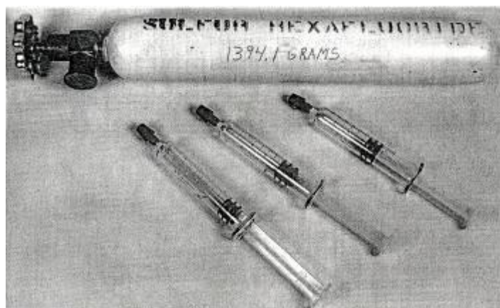
Fig. 1 Pressure bottle with SF_6 and syringes for samples
