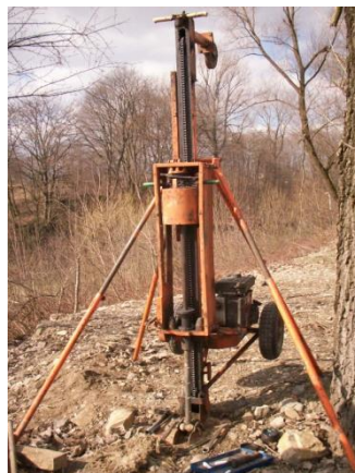
Fig. 3 Heavy dynamic penetration dig of the Borros system
