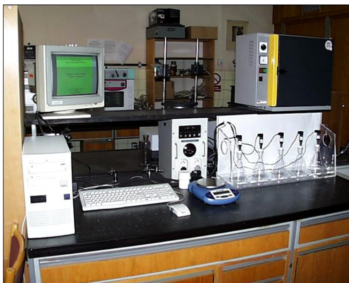
Fig. 8: Apparatus of isothermal sorption of oxygen at the VSB-Technical University of Ostrava
