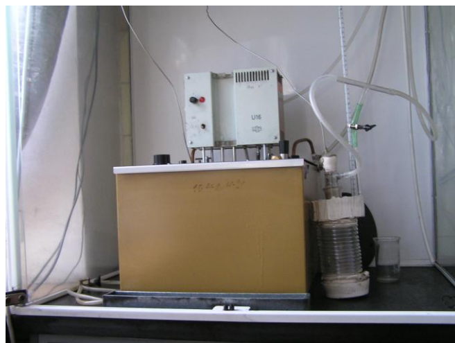
Fig. 4: U16 thermostat together with a reactor
