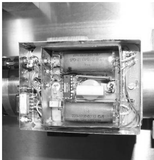
Fig. 2. Gerdien condenser design.
