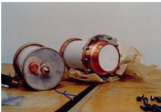
Fig. 5 Experimental construction of vircator, P_{\max} = 250 MW
