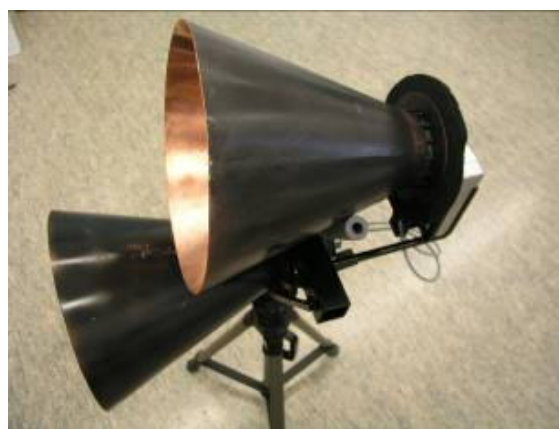
Fig.3. Realization of optimized combined calorimetric sensor
