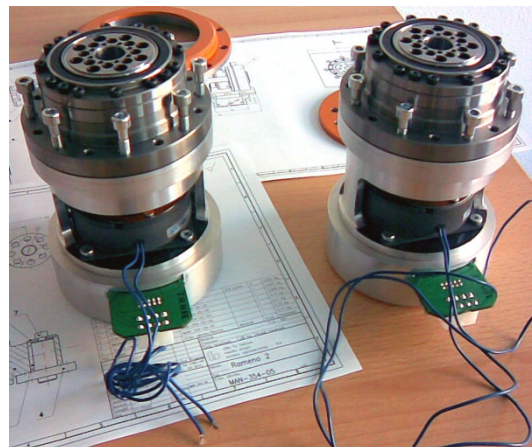
Fig. 4 Assembly of drive units
