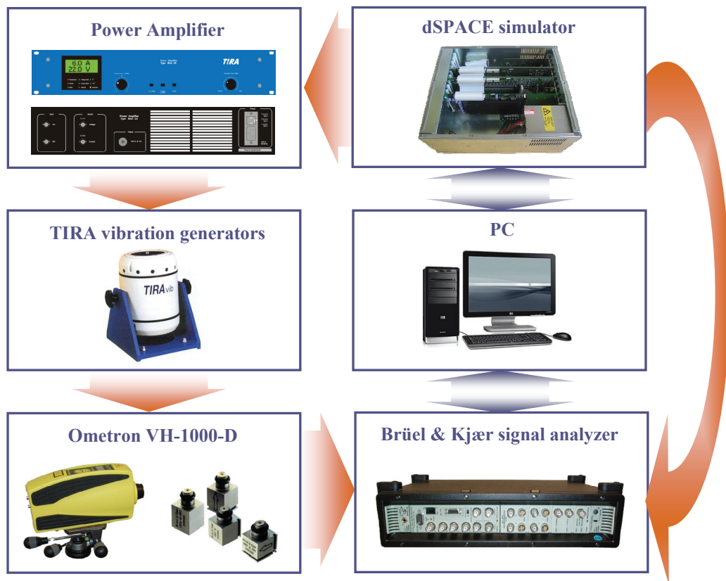
Fig. 8 Connection of hardware devices
