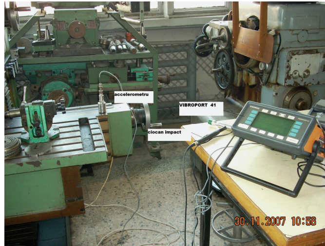
Fig.7 Vibroport 41 and the position of the accelerometer
