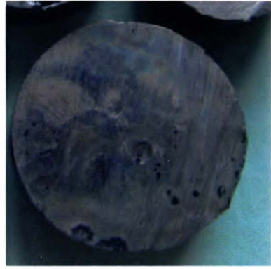
Fig. 4 Surface of solder (E14, Ø12) after salt spray test, exposition 240 h
