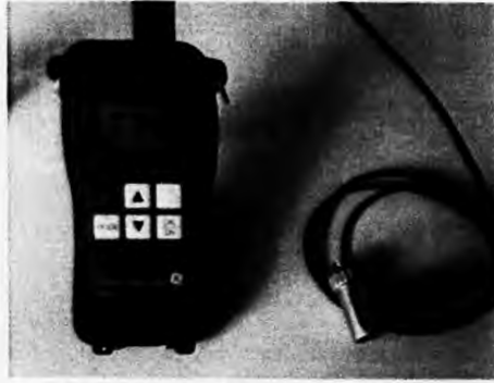
Fig. 1 GE DM4 ultrasonic thickness gauge
