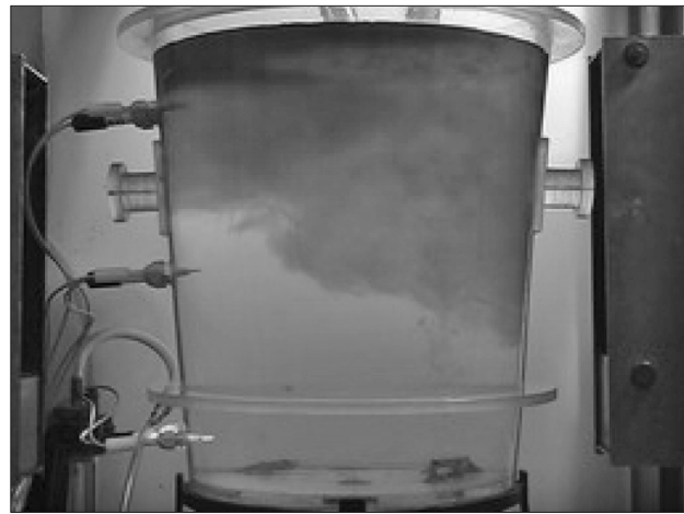
Figure 3. Red tracer visualisation (KMnO 4 ) of homogenisation process
