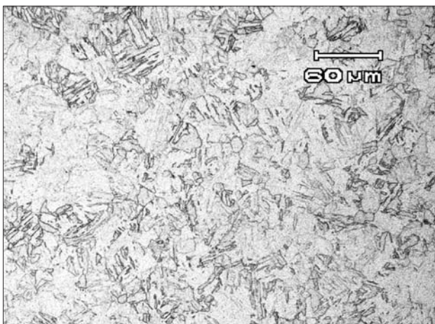
Figure 1. Microstructure of quenched steel X2CrNiMo 13-6-2
