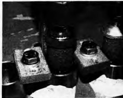
Fig. 2: The porous implant-bone substitute model fixation preparation for later push out tests
