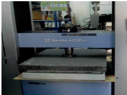
Fig. 3. Flexural test of concrete slabs.
