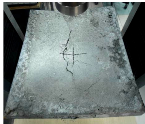
Fig. 11. Failure of steel fiber rubberized concrete (SFCR22.5)
