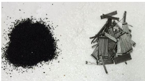
Fig. 1. Crumb rubber and steel fiber.
