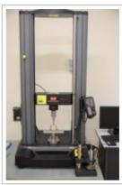
Instrument Name & Model: 5969 – 50kN Electro-Mechanical UTM
