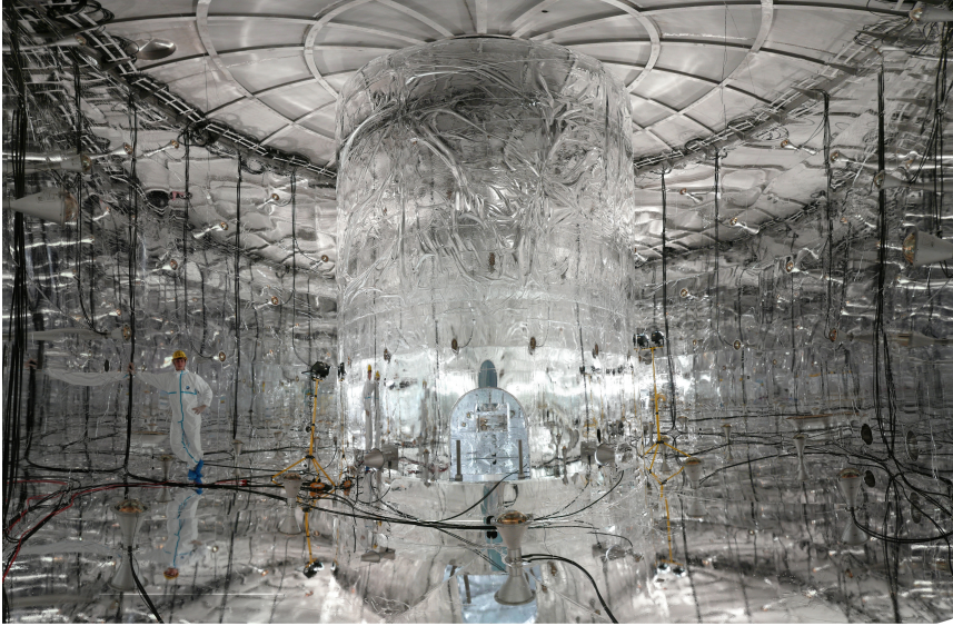
Figure 5: Inside the water tank after the installation of the muon veto system — August 2009, photo courtesy of Kai Freund (GERDA collaboration).
