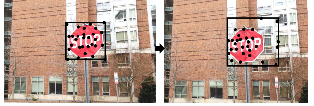
Figure 7: Tracked feature points deviate due to changes in the angle of the object.
