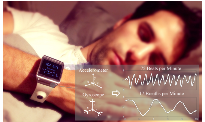
Fig. 1. We present a novel approach for measuring cardiac and respiratory parameters from wrist motions using a smart watch (Samsung Galaxy Gear), even when the wrist is not held against the chest.
