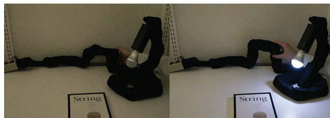
Figure 7. LineFORM used as a shape-changing cord which transforms into a lamp. A user can control its brightness through a rendered lever.
