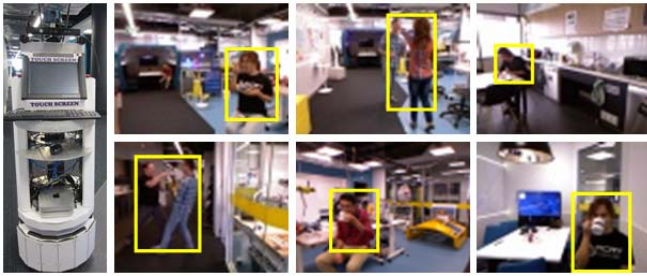
Figure 4. Samples of generated action region proposals and recognized scene and action label on our Guiabot robot dataset.
