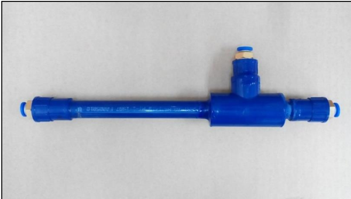
Figure 3: Fabricated Blue Model of RHVT using air as working fluid
