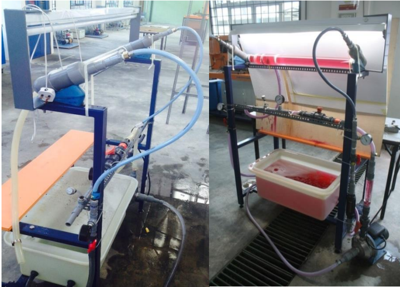
Figure 6: Experimental setup of flow visualization experiment
