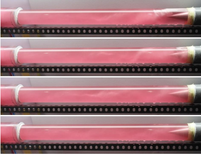
Figure 12: Flow visualization using syrup and bubble
