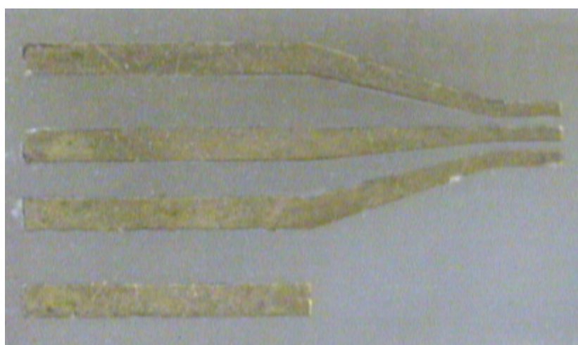
Figure 4: A Complete Fabricated Sensor for the Area Size of 1.04 mm 2 .
