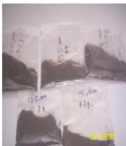
Figure 9: Different Size of Bladderwort Range from 75 to 600 \mu\text{m}
