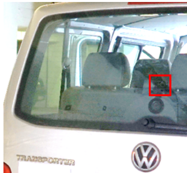
Figure 6: View onto the rear window pane of the test car. The rear environment camera (red rectangle) is looking at the area behind the car. Image brightness increased strongly for better visualization.
