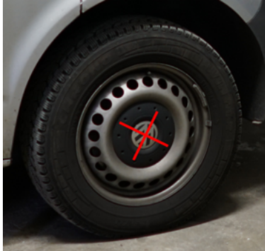
Figure 4: Rim centres (red cross) are used as ground control points for the transformation into the vehicle coordinate system. The emblem of the car manufacturer is often placed in the rim center providing a clear defined central point.
