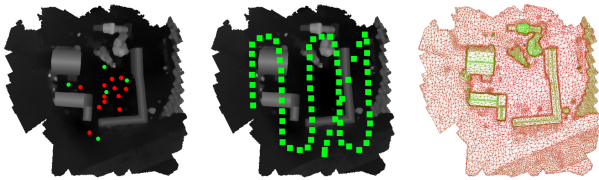
Figure 16. The UAV acquisition (Case 2). From the left: Distribution of GCPs (green) & CPs (red), acquisition protocol, initial mesh (from result of method 1) generated by MicMac.
