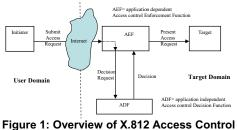
Figure 1: Overview of X.812 Access Control Function
