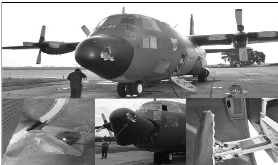
Photo 1. Damages caused by lightning on a military aircraft
