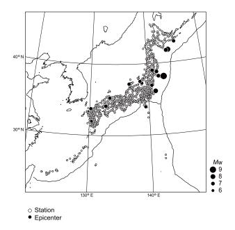
**Figure 2.** Station and epicenter map. Stations of seismic intensity meters (open circles) and epicenters of the events (solid circles) for which seismic records were used in this study are denoted.
