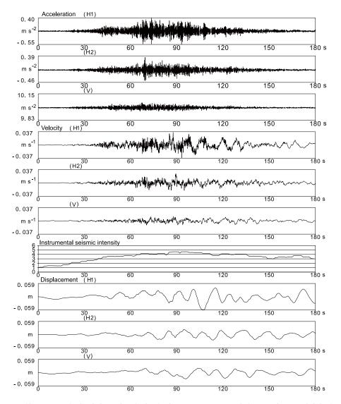
Figure 6. Seismic waves and instrumental seismic intensity obtained using prototype tsunami alarm equipment. Original acceleration records, velocity records for instrumental seismic intensity, instrumental seismic intensity, and displacement records are shown.
