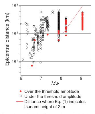
**Figure 3.** Data distribution of the maximum vertical displacement amplitude. Amplitude data which exceed the threshold value (0.081 m) are presented by red dots. The red line indicates the distance at which tsunami height is 2 m based on the Eq. (1) by Abe (1981).
