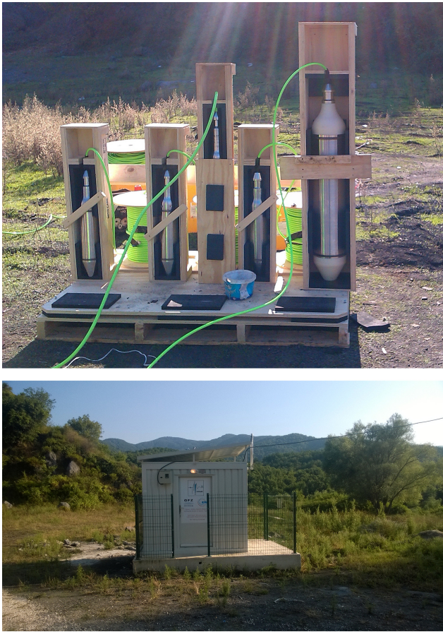
Figure 4. Upper part: GONAF downhole seismic instruments prior to deployment at the Kurtkoy station on the Armutlu Peninsula. The 300 m deep, gimbaled 1 Hz 3-C L4 seismometer sonde is on the right. In the middle is the combined 300 m deep 3-C 15 Hz DS200 and gimbaled 2 Hz HS-1 sonde. The other three sondes are the vertically distributed, gimbaled 1-C 1 Hz L4 seismometers. For redundancy each sonde has its own waterproof signal cable with an internal Kevlar stress member. Lower part: the 10 ft containers used to cover each station and to house the special low-noise Guralp CMG-DM recorders, telemetry systems, and their support equipment.
