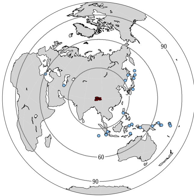
Figure 6. Epicentral distribution of teleseismic earthquakes used in the study (30–90°). Rectangles indicate seismic stations in this study.
