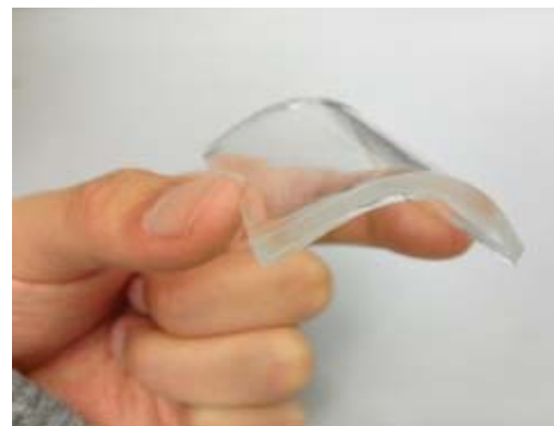
Fig. 2. Fabricated PDMS optical waveguide. The waveguide is elastic and flexible.
