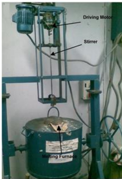
Figure 1: Electric resistance furnace used for fabrication of Al-SiC MMC
