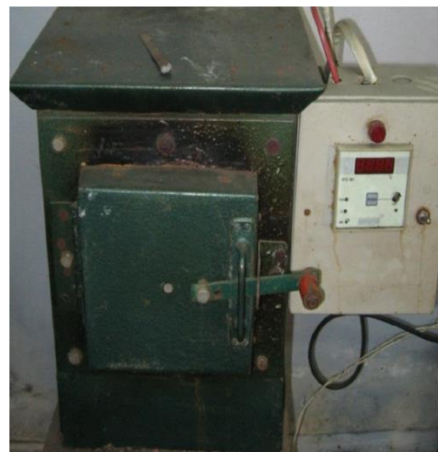
Figure 2: Box furnace used for pre-heating of SiC reinforcement.
