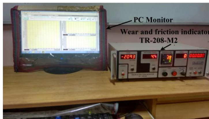
Figure 4: Wear and friction monitor attached to tribotester.
